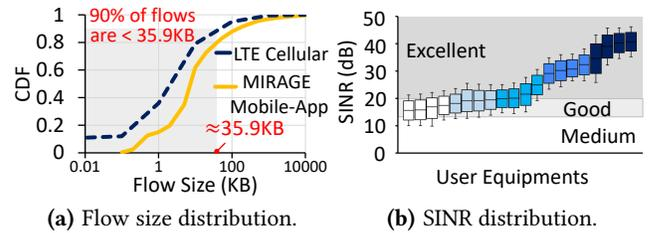
**Figure 2: Downlink cellular traffic distribution [41] and channel quality distribution across UEs in our evaluations.**
