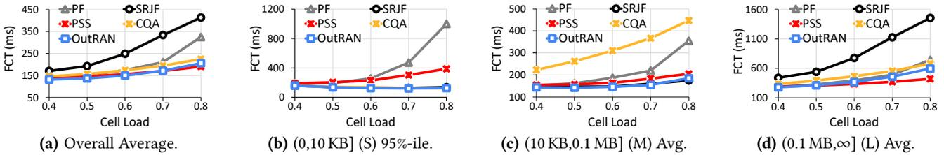
Figure 15: [NS-3 LTE] [61] FCT across different cell load in LTE under LTE cellular workload [41].
