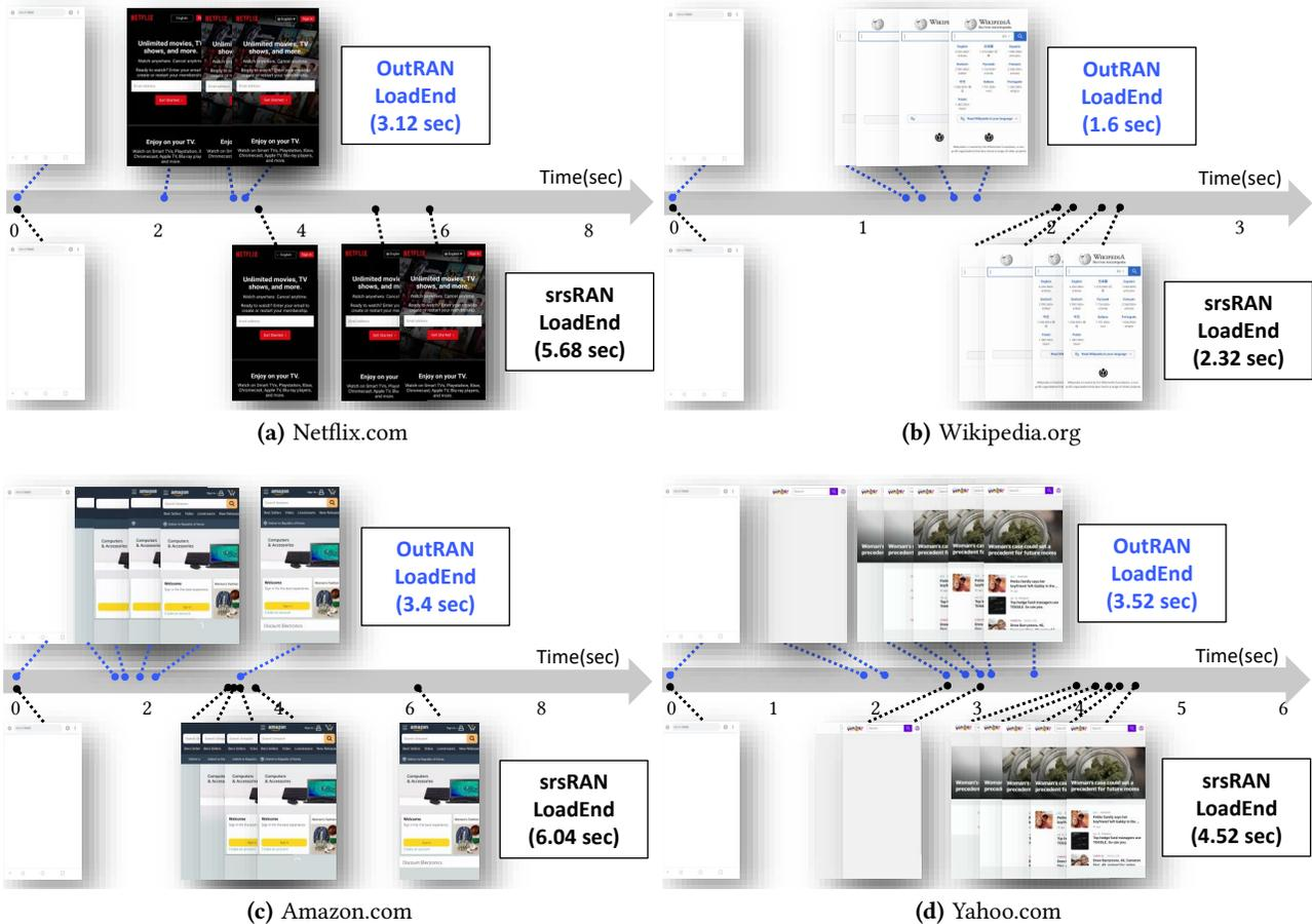
Figure 22: [Testbed] Comparison of Web Page Loading Time between OutRAN vs. srsRAN. The video is available at <https://ina.kaist.ac.kr/projects/outran>.
