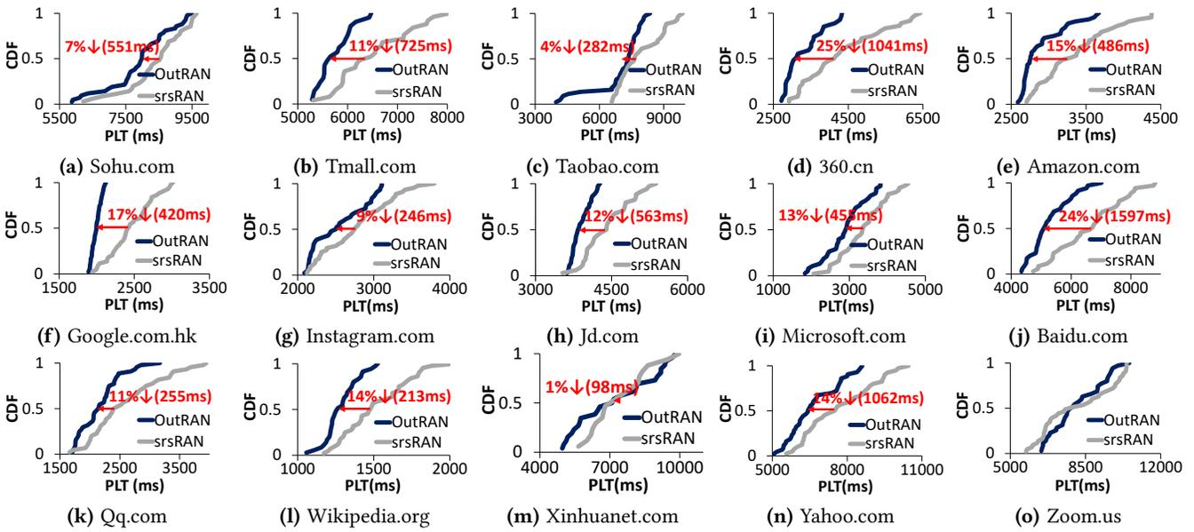
Figure 21: [Testbed] PLT across rest of the top 20 Webpages from Alexa.
