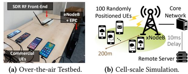
**Figure 11: Testbed and simulation topology.**
