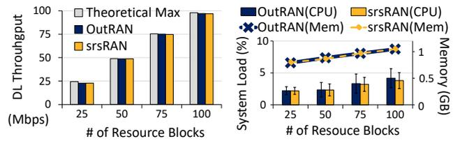
Figure 14: [Testbed] Scalability vs RBs.
