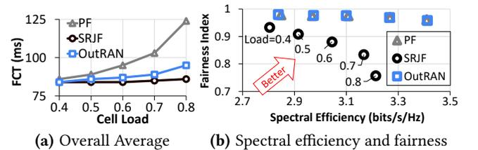
Figure 20: [NS-3 5G] [32] FCT across different cell load in 5G under 2019 mobile-app traffic [12].
