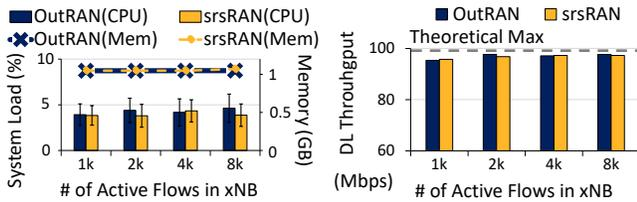
Figure 13: [Testbed] Throughput & resource usage.
